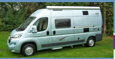
**Dimensions** Length - 5.998m Width - 2.05m Height - 2.65m Internal height - 1.90m
